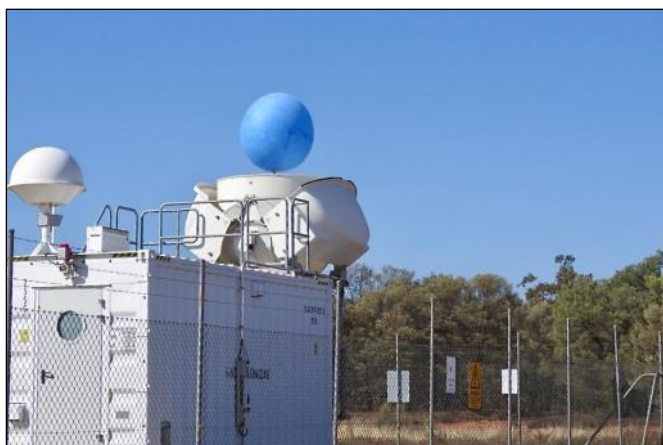
4. Weather balloon being automatically released at the Charleville Weather Station. (Graham Shaw).
