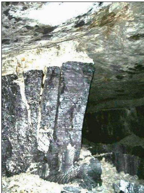
17. Expansion in a claystone roof (tuff) has warped the coal pillars. (Hayes, 2001).
