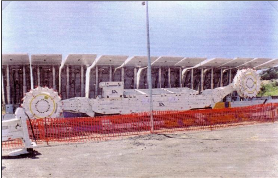
19. Continuous miner and roof supports used at the Moonee Colliery. (Photo from the ELMHS Collection).
