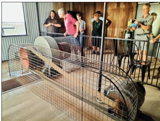
2. Pelton Wheel that turns from a flow of artesian water which then drives the generator. (Sue Rogers).
