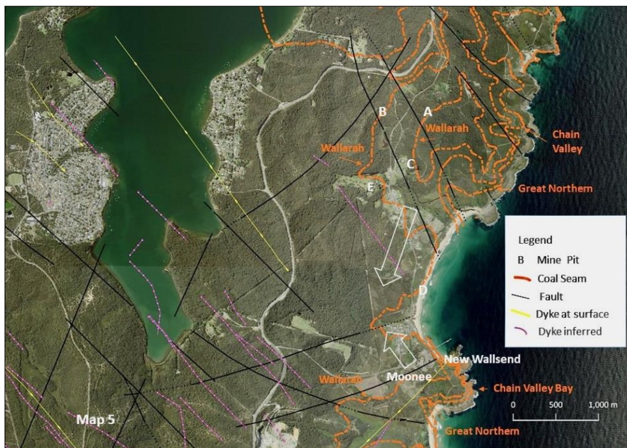
Map 5. Structural geology and coal seams at Catherine Hill Bay. The arrows show direction of dip. (Prepared by R Miller from NSW Seamless Geology and QGIS).
