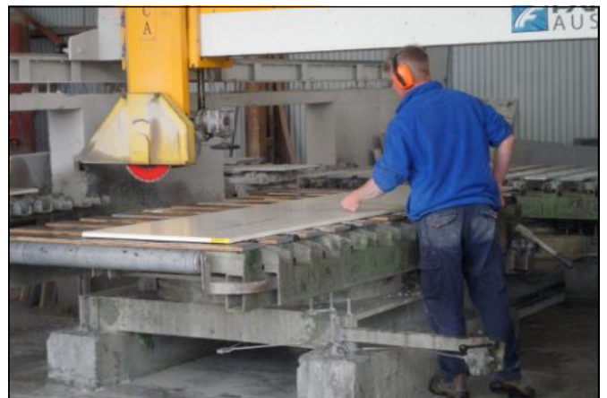
50. Trimming stone slabs at the Central West Granite Supplies.
