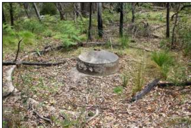
47. Chilean mill remnant - used to grind wolframite ore.
